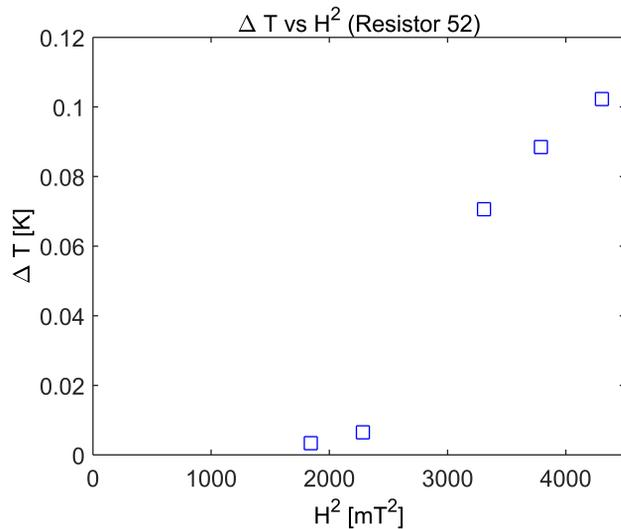
Figure 4: Heating in resistor near suspected quench area  $\Delta T$  plotted against the square of the magnetic field,  $H^2$ .
