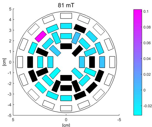
Figure 3: Example temperature map of the 500 °C sample at 1.6 K and a peak sample plate field of 81 mT. This localized heating, near the peak field ring 2.5 cm from the center, is indicative of a defect quench.
