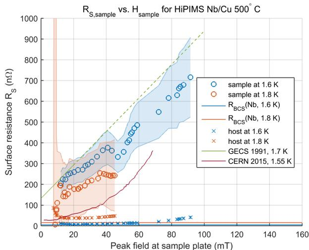
Figure 2: Surface resistance of the 500 °C sample at 1.6 K and 1.8 K, compared with the surface resistance of the body of the cavity as well as the BCS prediction of  $R_s$  for niobium at 3.9 GHz. Also included are previous results of sputtered films, scaled to 3.9 GHz. Results in green from LEP2 cavities measured for GECS and presented in [5]; more recent HIPIMS results in maroon presented in [6].
