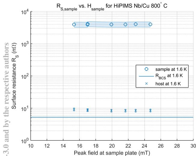
Figure 5: Surface resistance of the 800 °C sample at 1.6 K, compared with the surface resistance of the body of the cavity as well as the BCS prediction of  $R_s$  for niobium.
