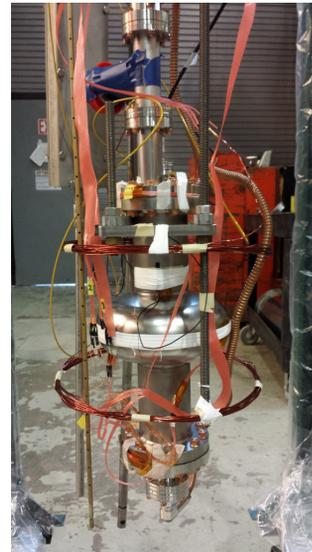
Figure 2: Experimental apparatus to measure the effects of trapped flux on cavity performance. A single-cell 1.3 GHz ILC shaped cavity was surrounded by a Helmholtz coil and dressed with fluxgate magnetometers on the iris and temperature sensors on the equator and both flanges.
