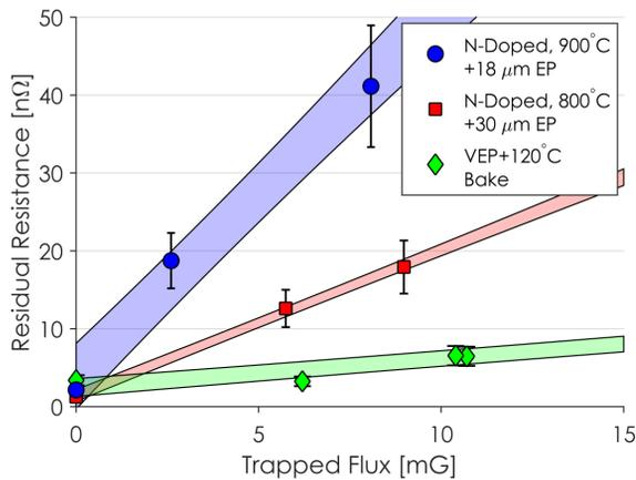
Figure 3: Residual resistance versus trapped magnetic flux for three of the cavities tested.  $R_{res}$  increases linearly with trapped flux and there is a large spread in slopes.
