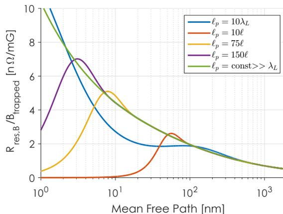
Figure 1: Residual resistance from trapped flux normalized to the amount of trapped flux as predicted by the Gurevich theory [4] for different interpretations of the mean spacing between pinning sites.
