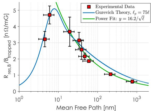
Figure 4: Sensitivity of residual resistance to trapped magnetic flux ( $R_{res,B}/B_{trapped}$ ) versus mean free path for the cavities tested. Also shown in a fit to the Gurevich theory assuming a linear relationship between mean free path and mean spacing between pinning sites. The only fit parameter is the constant of proportionality between these quantities.
