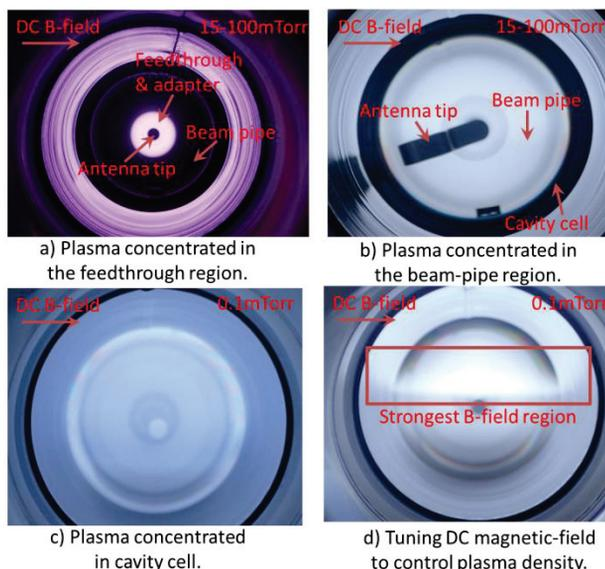
Figure 3: The summary of observed plasma ignited at different conditions.
