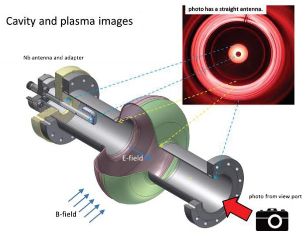
Figure 1: The schematic of plasma cleaning set-up. The up-right subplot shows an image observed from the view port.
