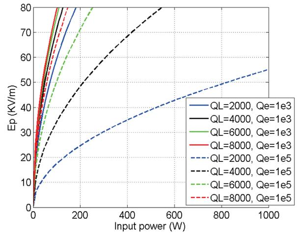
Figure 6: The peak electric-fields versus the input power at different  $Q_L$  and  $Q_e$ .
