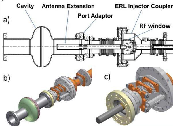
Figure 4: The new design of the coupler and cavity: a) 2D drawing of the coupler design connected to the cavity; b) 3D model of the coupler design; c) The details of the antenna extension of the coupler.
