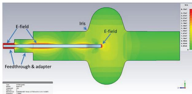
Figure 2: The Simulation of electric-field distribution of a 1.3GHz single-cell SRF cavity with a coupler.
