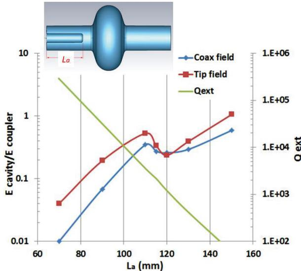
Figure 5: The curves of the ratio  $E_{coupler}/E_{cavity}$  versus insert depth  $L_a$  as well as the external Q versus  $L_a$ .
