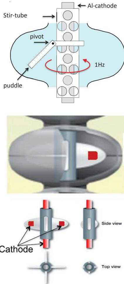
Figure 2: Top: Cornell cathode, Middle: Marui's i-cathode Ninja type-1, Bottom: retractable wings on Ninja cathode type-I.
