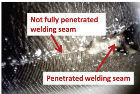
b) An inspection image of equator region indicates the unpenetrated welding seam.
