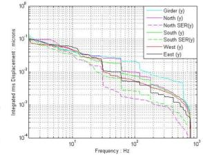
Figure 5: Enclosure vertical integrated rms displacement.
