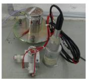
Figure 3: HLS, tri-axial geophone and seismometer.
