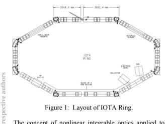
Figure 1: Layout of IOTA Ring.
