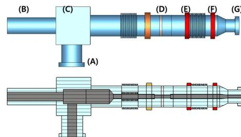
Figure 2: RISP 2<sup>nd</sup> prototype HWR coupler Type B. (A) RF power input. (B) Air-cooling line. (C) Transition Box (T-box). (D) RF window section. (E) 40 K thermal intercept. (F) 4.5 K thermal intercept. (G) Cavity port.
