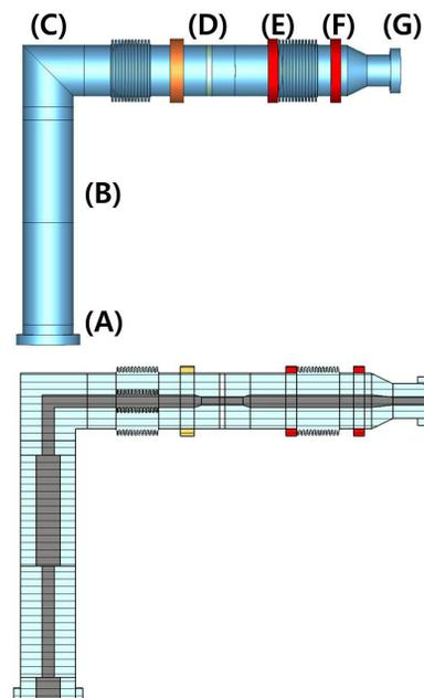
Figure 1: RISP 2<sup>nd</sup> prototype HWR coupler Type A. (A) RF power input. (B) Impedance matching section. (C) Elbow section. (D) RF window section. (E) 40 K thermal intercept. (F) 4.5 K thermal intercept. (G) Cavity port.
