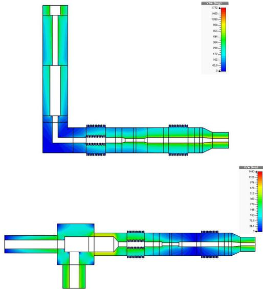
Figure 3: HWR coupler EM simulation. The upper figure shows the electric field distribution for the type A coupler and the lower figure represents the electric field for the type B coupler.
