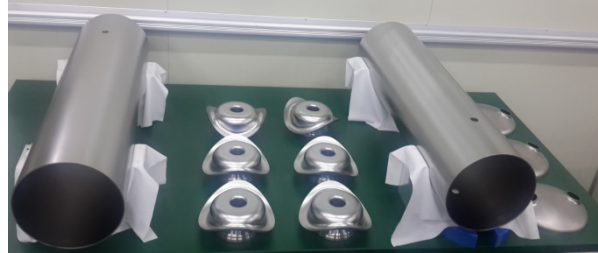
Figure 1: Formed parts of QWR cavities.
