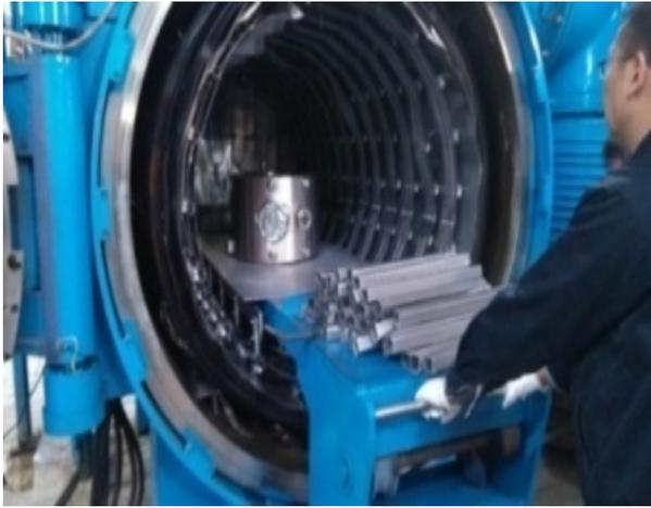
Figure 2: High temperature annealing facility.
