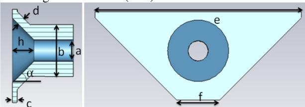
Figure 4: The dimension parameters of the transition structure.
