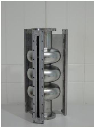
Figure 2: Niobium slotted cavity.
