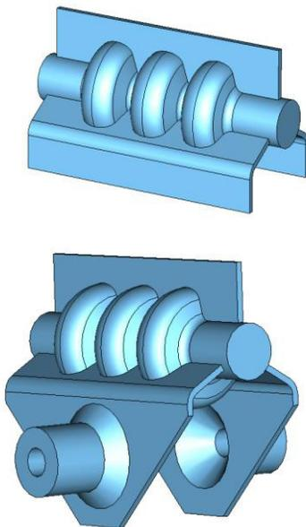
Figure 3: The slotted cavity with HOM extracting structure. Up: slotted cavity with rectangular waveguide (RW). Down: slotted cavity with rectangular waveguide to coaxial waveguide structure (WC).
