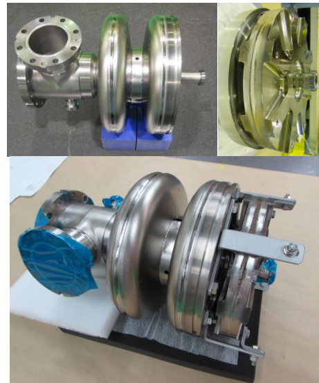
Figure 9: (upper left) First prototype cavity (upper right) Coke structure (bottom) Modification cavity.
