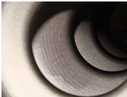
Figure 4: Inside cavity after hydroforming.
