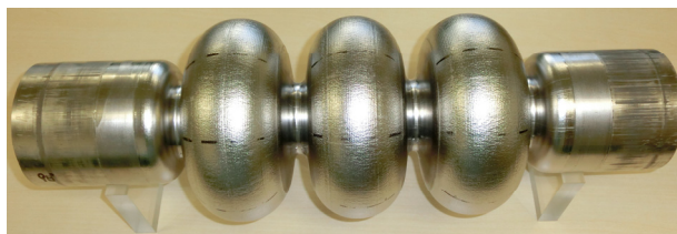
Figure 3: Niobium tube just after hydroforming.
