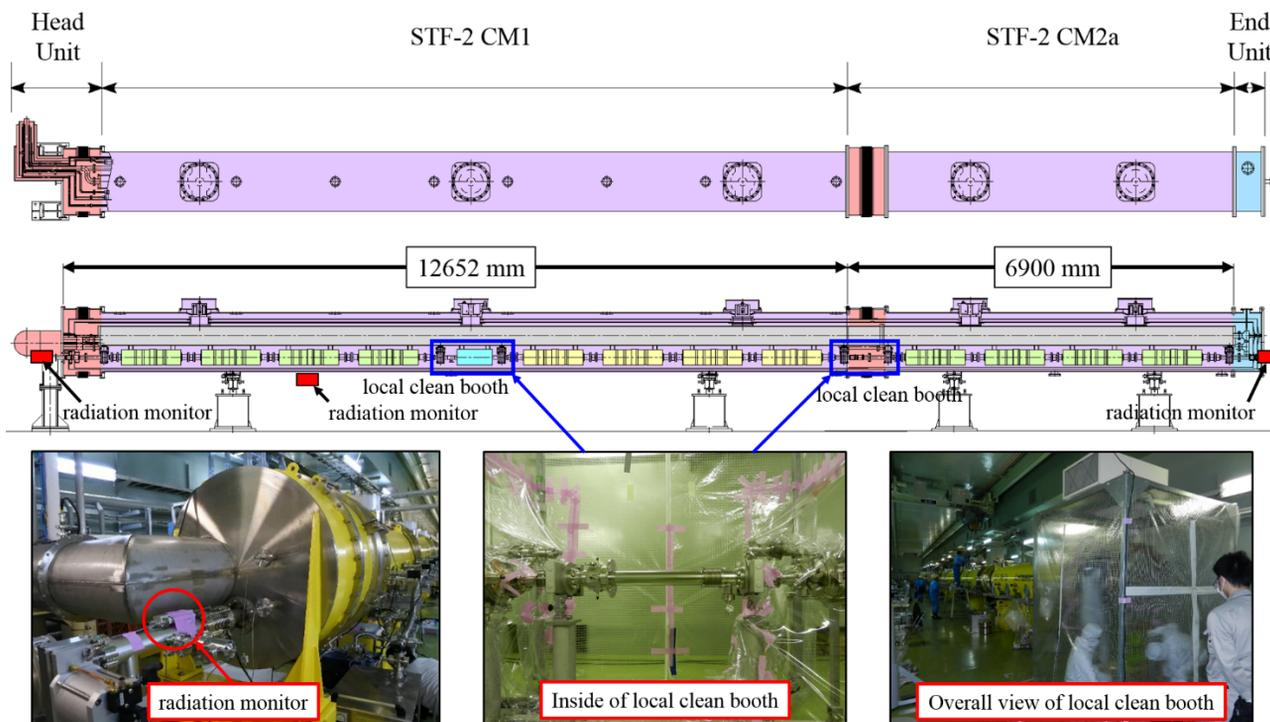
Figure 3: Schematic views of STF-2 cryomodule (top), location for radiation monitor at upstream of cryomodule (bottom left), and local clean booth in tunnel (bottom centre and right). In the top figure, three red filled squares show the locations for radiation monitor. The local clean booth was used for the connection of each cavity string in the tunnel, shown as two blue squares.
