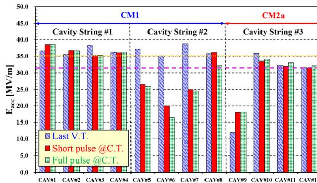
Figure 4: Cavity performance in STF-2 cryomodule. The dotted line at 35.0 MV/m and dashed line at 31.5 MV/m show the ILC specification in V.T. and C.T., respectively.
