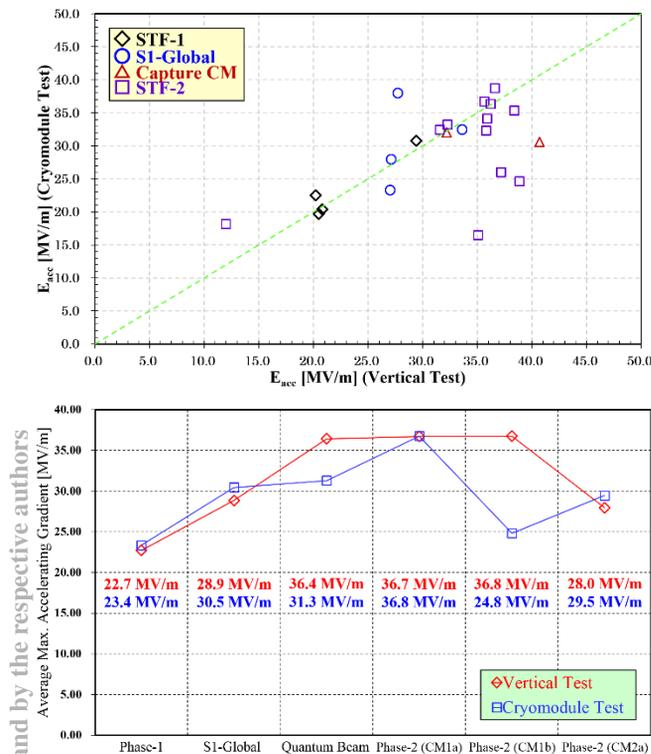
Figure 6: Comparison of cavity performance between V.T. and C.T. (top), and average gradient as each cavity string with four cavities (bottom). Quantum Beam cryomodule (Capture CM) has only two cavities. There are totally four degraded cavities, one in Capture CM and the others in STF-2. There was no performance degradation for Phase-1, S1-Global, CM1a and CM2a in Phase-2.
