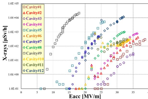
Figure 5: Radiation level measured at beneath cryomodule. Cavity #6 had quench by enormous heat loss.
