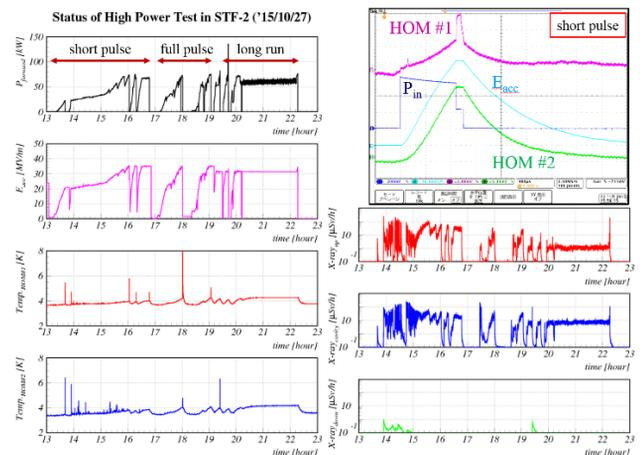
Figure 2: Trend graphs for forwarded power, accelerating gradient, and heating at both HOM couplers during RF processing by short and full pulse in cavity at 2K (left), one shot at unusual output from HOM coupler #1 in oscilloscope (right up) and x-rays measured at three locations near cryomodule (right down).
