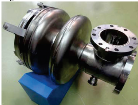
Figure 7: Picture of the prototype cavity at 4 th vertical test
