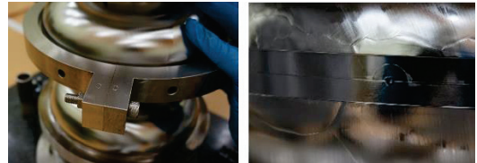
Figure 6: Equator with supporting jig (left) and equator after spot welding (right).
