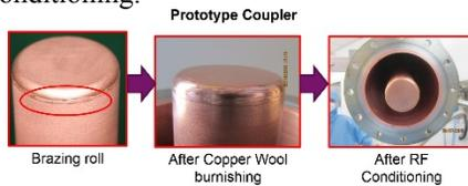
Figure 5: Example of surface finishing result.
