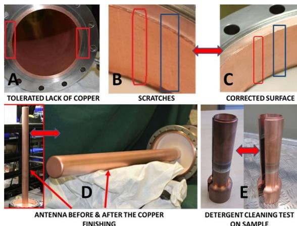
Figure 4: Copper plated surface finishing and cleaning.
