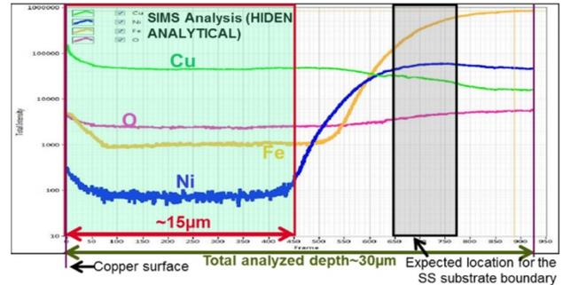
Figure 7: SIMS analysis of a copper plated stainless steel (SS) sample.
