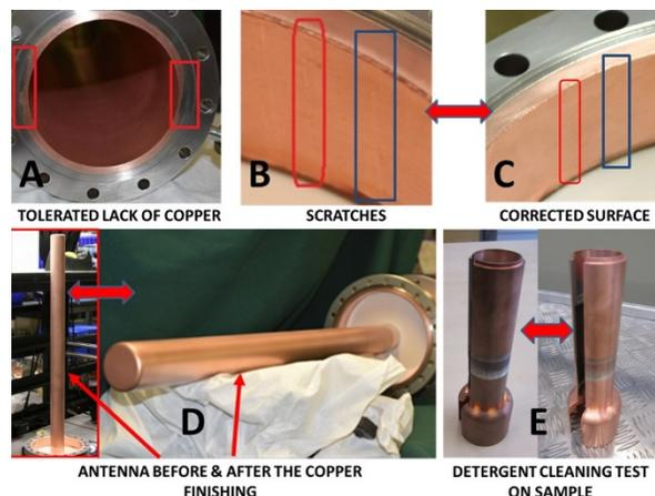
Figure 4: Copper plated surface finishing and cleaning.
