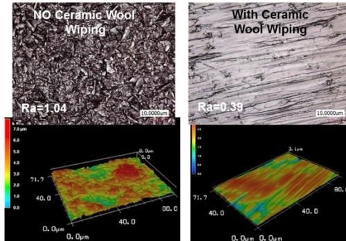
Figure 6: Ceramic wool wiping on copper plated surface.
