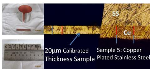
Figure 3: Copper plating thickness measurements.
