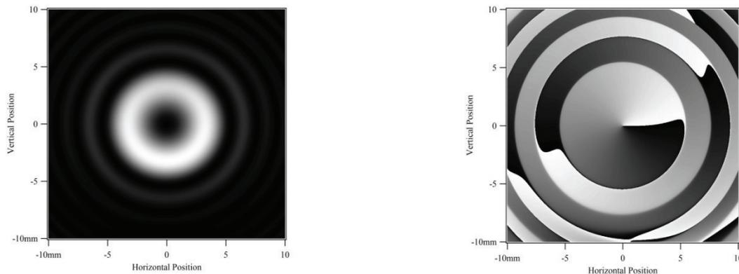
Figure 1: Calculated intensity (left) and phase (right) distribution of 2nd harmonics from a helical undulator. The calculation is done using SRW, under condition of  $\lambda = 355$  nm,  $\lambda_u = 88$  mm,  $\gamma = 978$ , and  $K = 3.8$ .
