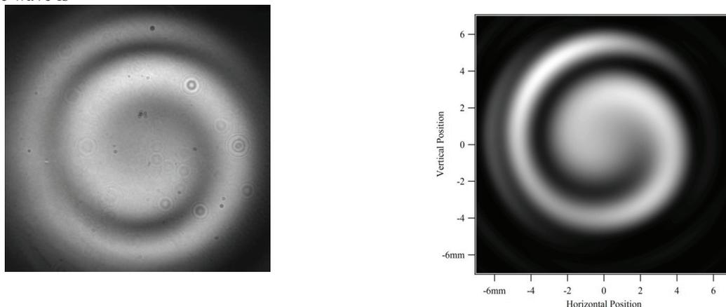
Figure 2: Measured (left) and calculated (right) spiral pattern from double undulator interference.
