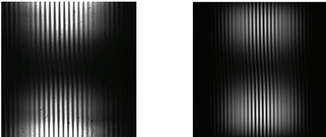
Figure 3: Measured (left) and calculated double slit pattern from 2nd harmonic radiation.
