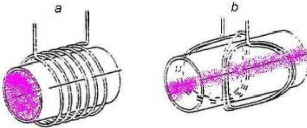
Figure 11: RF plasma generator antennae;
