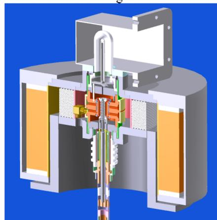
Figure 9: 1497 MHz klystron design.
