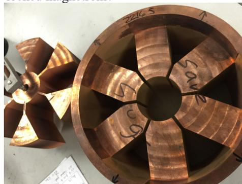
Figure 10: Anode structure for a 350 MHz magnetron.
