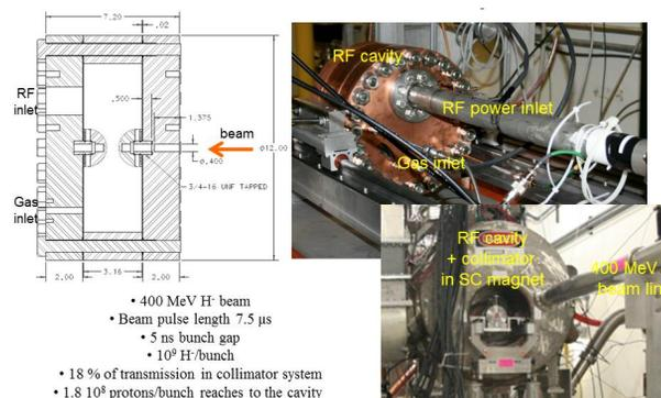
Figure 2: Beam tests of a GH2 pressurized RF cavity in a 5 T magnet at the Mucool Test Area at Fermilab.
