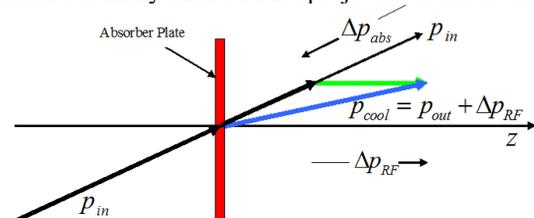
Figure 1: Principle of Ionization Cooling.
