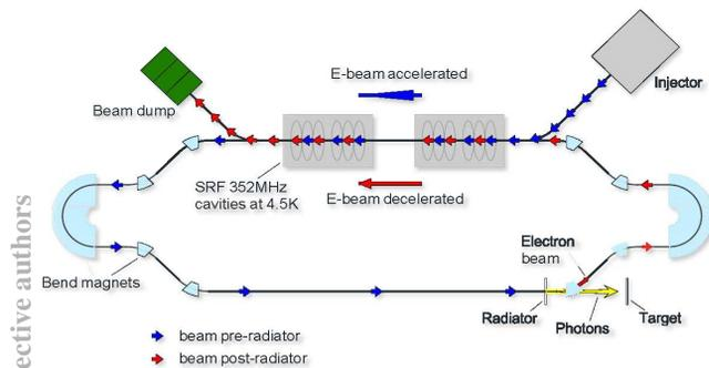
Figure 12: ERL to produce radioisotopes.
