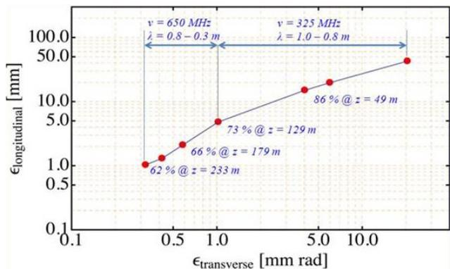
Figure 6: Muon beam emittance and survival evolution for a HCC as simulated using G4beamline.
