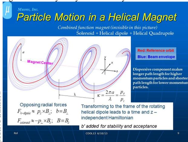
Figure 4: Particle motion in a Helical Cooling Channel.
