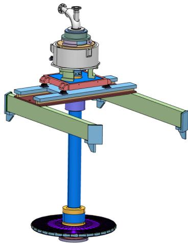
Figure 8: The ESS rotating target concept.
