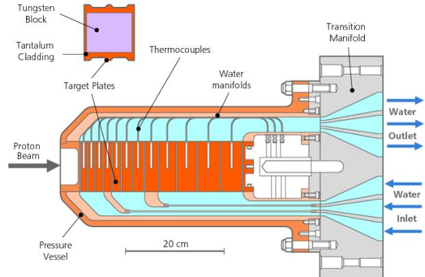
Figure 3: ISIS stationary solid target schematic.
