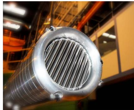
Figure 4: The SINQ Cannelloni target.
