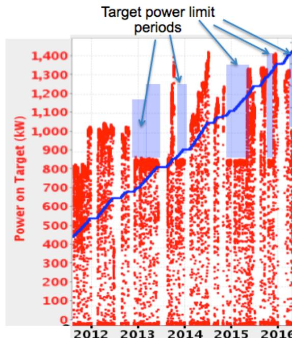
Figure 1: SNS Operational beam power, with periods limited by target concerns indicated in blue.
