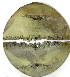
Figure 6: Representative cavitation induced damage on the inside wall of an SNS target vessel.
