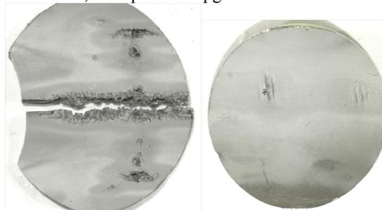
Figure 7: SNS target samples for nominal target (left) and jet flow (right).
