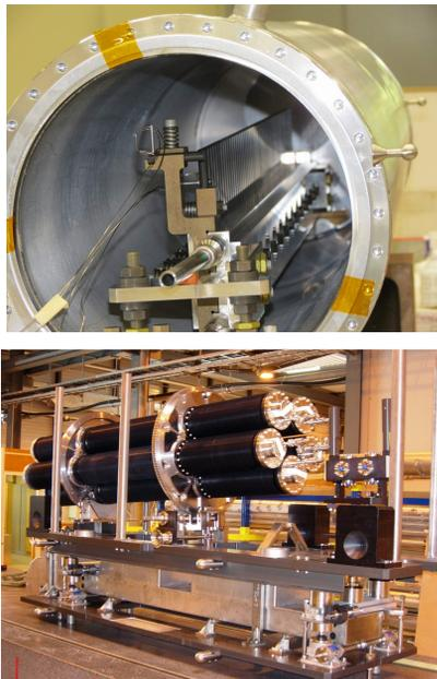
Figure 9: NOVA (top) and CGSN (bottom) neutrino targets.
