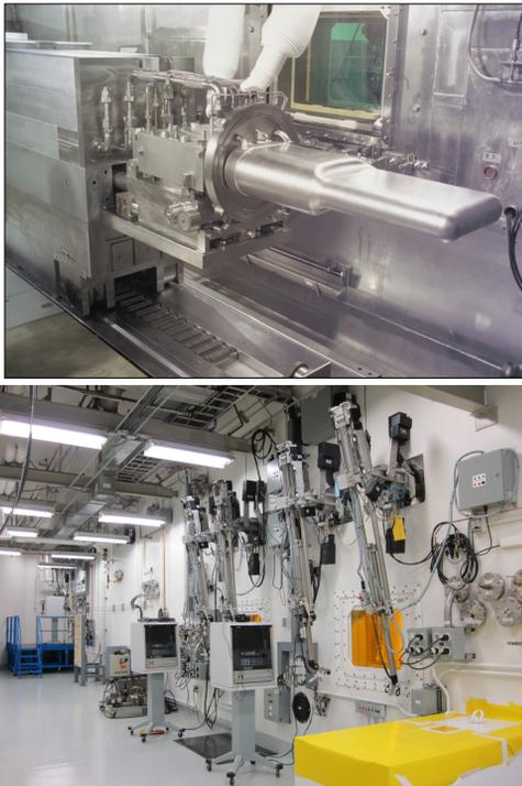
Figure 2: A target assembly inside the SNS hot-cell (top) and a view of the hot-cell outside (bottom) with manipulator equipment.
