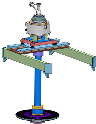
Figure 8: The ESS rotating target concept.
