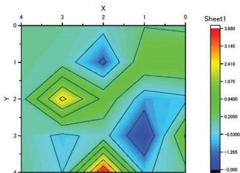
Figure 4 (b): <sup>208</sup>Pb distribution image reconstructed by the transmission of 5292-keV NRF peaks including atomic absorption.
