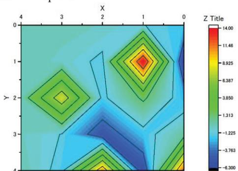
Figure 4 (c): <sup>208</sup>Pb distribution image reconstructed by the transmission of 5292-keV NRF peaks.
