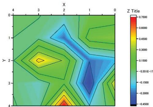
Figure 4 (a): Atomic absorption image measured by the LaBr<sub>3</sub>(Ce) detector
