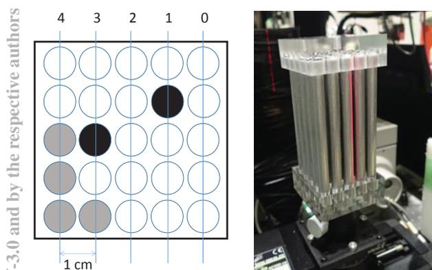
Figure 2 Left: Top-view of the  $5 \times 5$  array sample. Black circles are natural lead rods, Grey circles are stainless steel rods, and white circles are aluminium rods. Right: Photo of the sample with moving and rotating stages.
