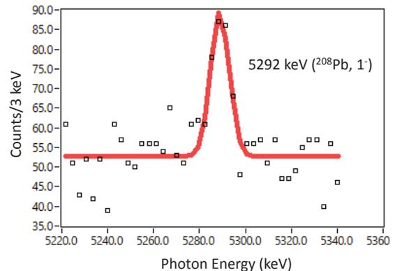
Figure 3 Upper: Typical spectrum from the witness target measured by Ge. Lower: Expanded spectrum of ROI around 5292 keV with a Gaussian peak fitting result. The peak width of about 4 keV was obtained.
