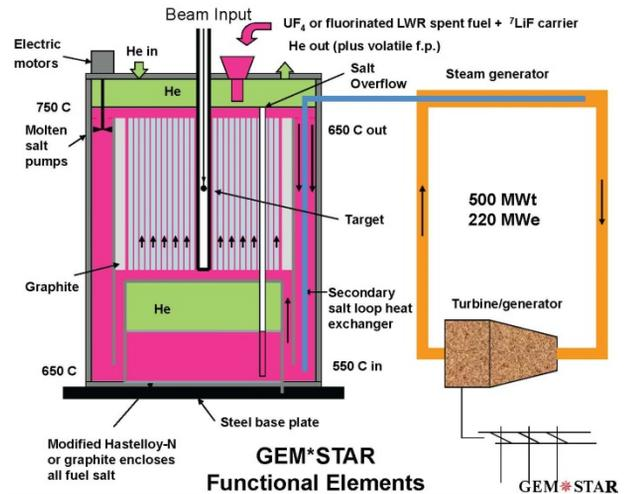
Figure 2: Cross-sectional view of GEM\*STAR reactor driving an external generator.
