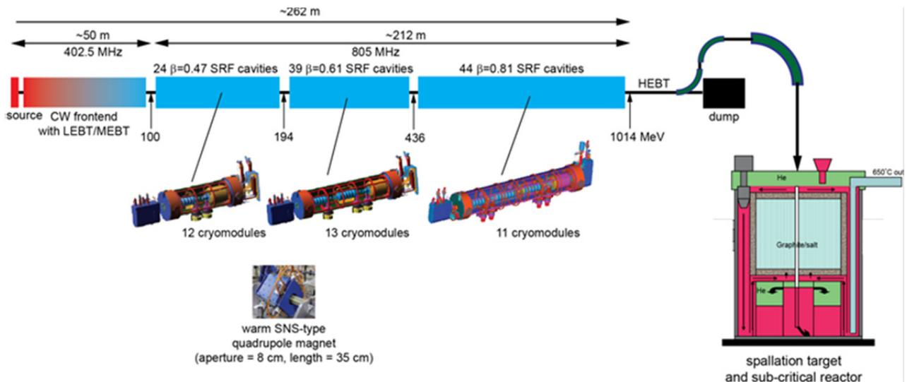
Figure 3: Configuration of a GEM\*STAR reactor driven by a cost-reduced version of the ORNL SNS 1014 MeV proton accelerator (not to scale). HEBT denotes high energy beam transport (HEBT). An accelerator of this type could support up to four GEM\*STAR reactors in the plutonium disposition application.
