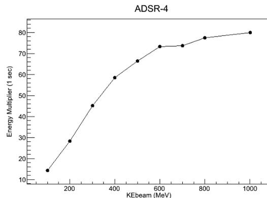
Figure 5: The energy multiplier is calculated using beam from G4beamline[6] and reactor simulation in MCNP 6.1, then plotted vs. the proton beam energy. This was generated with the software tool MuSim, described below.
