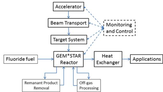
Figure 1: Block diagram showing major elements of the GEM\*STAR system.
