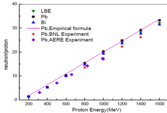
Figure 4: Neutron production per incident proton as a function of proton energy for targets 10 cm diameter by 60 cm long for data and FLUKA simulations [4].
