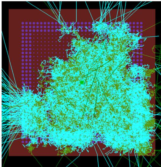
Figure 6: MuSim simulation of neutrons and gammas produced by a single 1 GeV proton on a U target in the GEM\*STAR reactor. Neutron tracks are green and gamma tracks are cyan. Graphite elements are shown in brown and the molten fuel mixture of LiF and  $\text{UF}_4$  in the tubes is shown in blue. The core is shown in 50% transparency to better visualize the tracks throughout the core.
