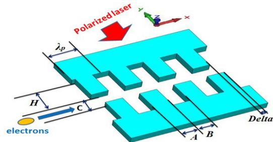
Figure 1 : Schematic of a dual-grating structure.
