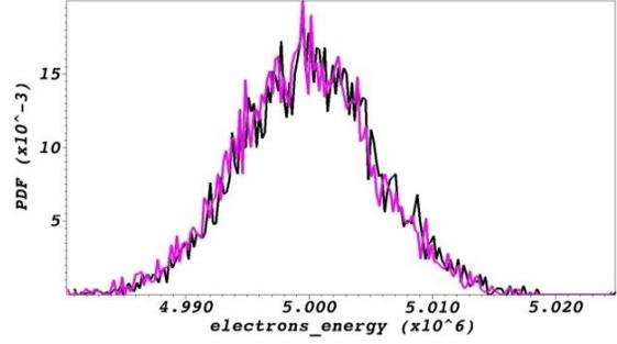
Figure 5 : Bunch energy distribution at time t=0 (black line), and t= structure exit (pink line) without a laser, where PDF stands for probability density function.
