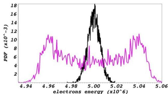
Figure 8: The bunch energy distribution at time  $t=0$  (black line), and  $t=\text{structure exit}$  (pink line) after interaction with the laser.
