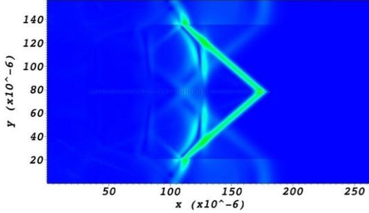
Figure 3 : The electric field of the electron bunch traveling along the vacuum channel of the structure.
