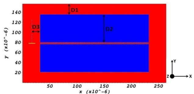
Figure 2 : Model of a 100-period dual-grating structure in the VSIM code. The red area represents vacuum, the blue area dielectric material with a refractive index  $n=1.5$ , and the injected electron bunch is represented in yellow.
