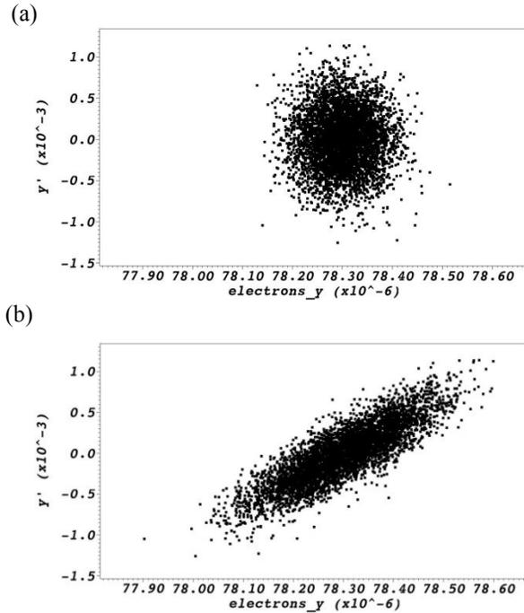
Figure 4: Transverse (y direction) phase space for the electron bunch at time t=0 (a), and t= structure exit (b)
