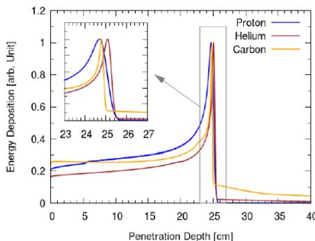
Figure 1: [3] A comparison of the Bragg peak for a specific penetration depth for protons, helium ions and carbon ions. The Energy deposition is relative to the maximum deposition for the ion species. A larger fragmentation dose occurs from carbon ions, in comparison to helium ions and protons.
