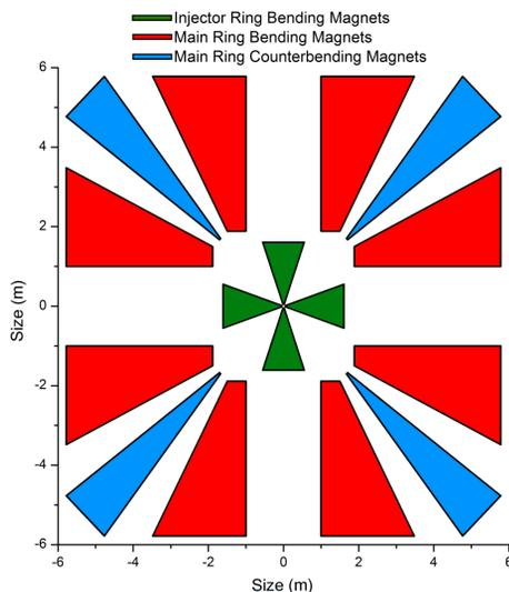
Figure 3: A representation of the magnet layout for the helium nsFFAG. The injector ring is highlighted in green and the main ring in red and blue. The blue magnets are counterbend magnets. All other magnets are bending magnets
