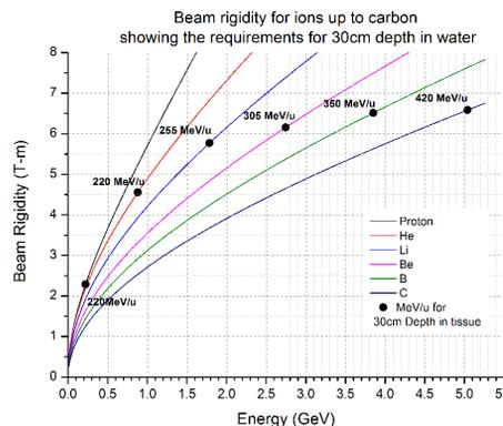
Figure 2: The beam rigidity required to bend the beam for varying kinetic energy for fully stripped ions up to carbon. The beam rigidity required to reach 30cm water depth is highlighted for each ion, and labeled with the energy required per nucleon.
