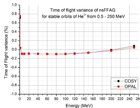
Figure 4: A graph showing the time of flight (ToF) variance compared to the mean against kinetic energy for helium in the injector ring. Results are shown from two different codes, COSY and OPAL.
