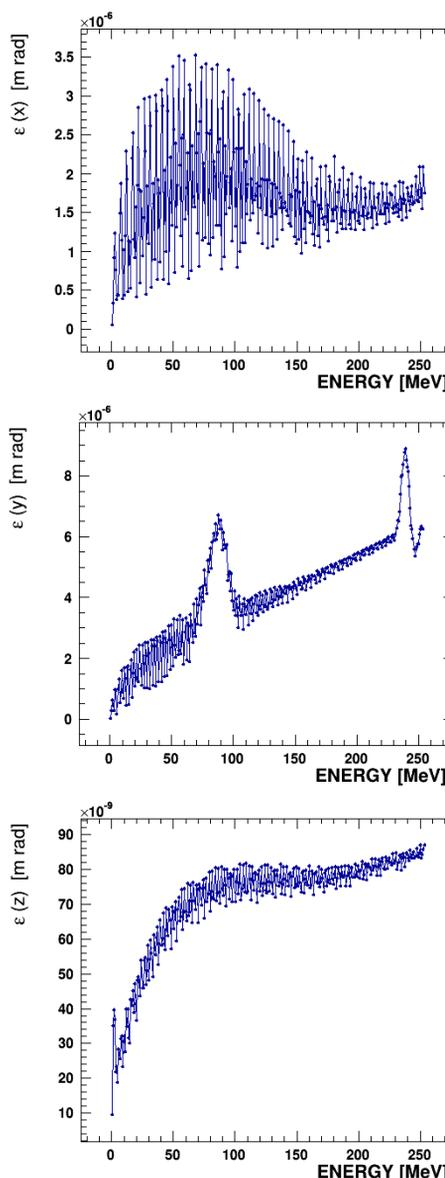
Figure 6: The RMS emittances without space charge from top to bottom for x, y and z respectively. The peaks in the y emittance are due to the non-perfect isochronicity which are caused by OPAL and should be ignored.
