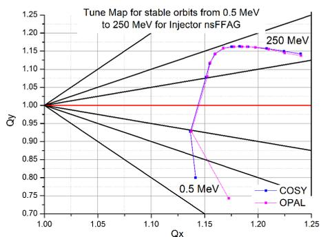
Figure 5: A tune map showing the tunes provided from COSY and OPAL. It can be observed the vertical tune crosses an integer resonance. This tune suppression is caused by the overlapping fringe fields near at the inner radius.
