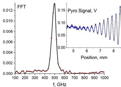
Figure 4: FFT of the raw experimental interferogram (inset) obtained at  $0.96^\circ$  pitch angle of the radiator, 2.5 MeV beam kinetic energy and 11.3 A current in the alpha-magnet.
