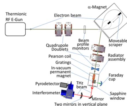
Figure 1: Schematic layout of the experimental setup. Five beam steering correctors are not shown. The layout footprint is about  $(1 \times 1.5) \text{ m}^2$ .
