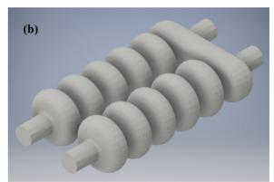
Figure 1: (a) Schematic of source of coherent radiation driven by SCRF dual axis asymmetric ERL. (b) Layout of dual axis asymmetric cavity for ERL.
