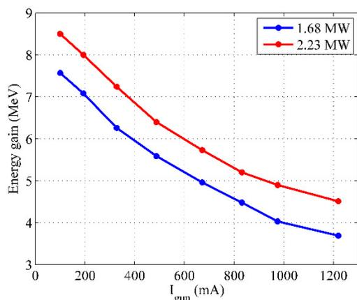
Figure 4: The average energy gain in the high power test.
