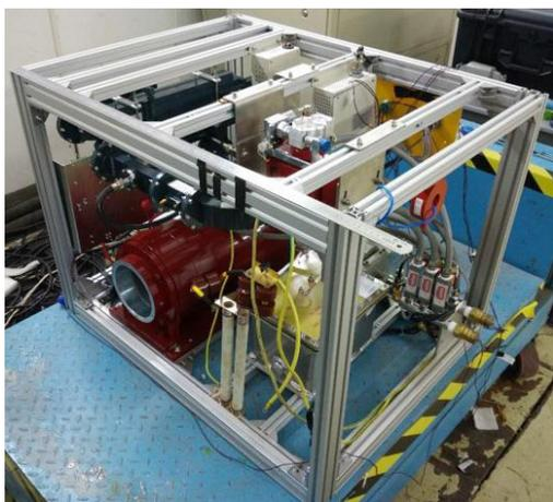
Figure 2: The C-band 4/8 MeV dual-energy accelerator.
