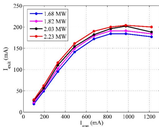
Figure 3: The pulsed current at the gun exit in the high power test.
