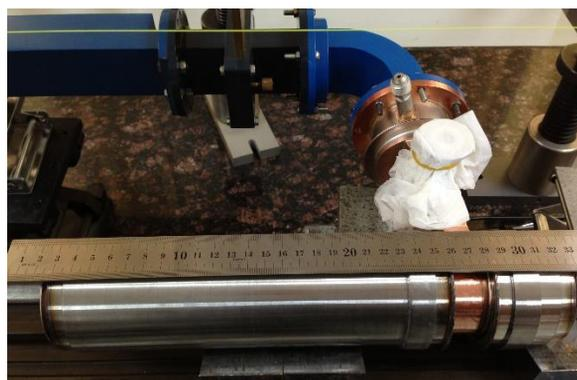
Figure 1: The C-band 6 MeV accelerating structure prototype II.
