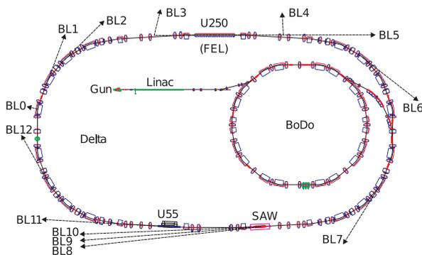
Figure 1: Overview of the DELTA facility including the storage ring and its booster synchrotron BoDo.
