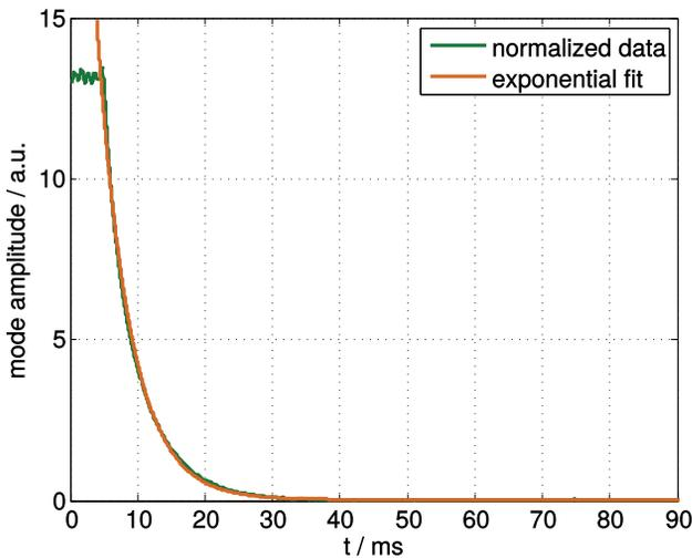
Figure 2: Exponential fit to determine damping rate of the most unstable mode of DELTA (no. 12) at a beam current of 39.3 mA to  $1/\tau = 0.207 \text{ ms}^{-1}$
