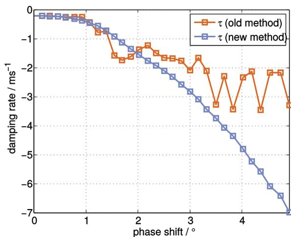
Figure 4: Damping rate of mode 12 as a function of the phase shift of the RF phase modulation at a beam current of around 39 mA. The old method, using exponential fits (orange curve), only works for small phase shifts. The new method, using the saturation value (blue curve), works for the whole regime.
