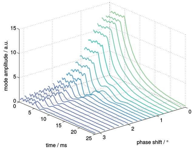
Figure 3: Mode signals of mode 12 at approx. 39 mA while the modulation amplitude is swept. Different modulation amplitudes are color coded increasing from green to blue.
