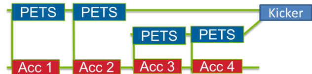
Figure 5: Full staging TBA layout. This beamline will be installed after kicker design and fabrication is complete.
