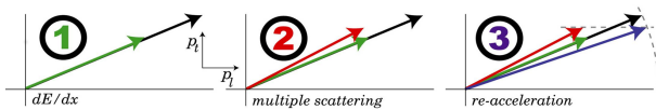
Figure 1: Principle of ionization cooling: 1) The overall momentum is reduced through ionization where \langle \frac{dE}{dx} \rangle is the mean energy loss of the muons. 2) Transverse momentum increases through multiple scattering. 3) Through re-acceleration, longitudinal momentum is regained.
