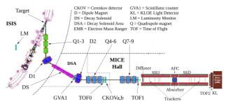
Figure 2: Plan view of MICE Step IV configuration, beginning from the target in ISIS.
