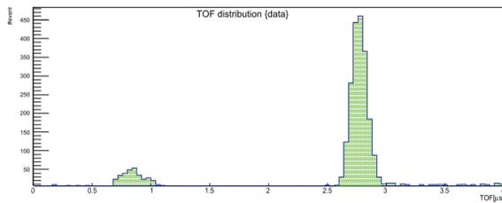
Figure 3: Event timing distribution observed by the MCP detector.
