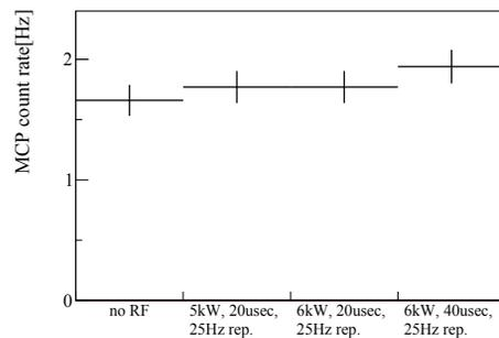
Figure 6: Result of the MCP background measurement. All the measurements are consistent each other within statistical error.
