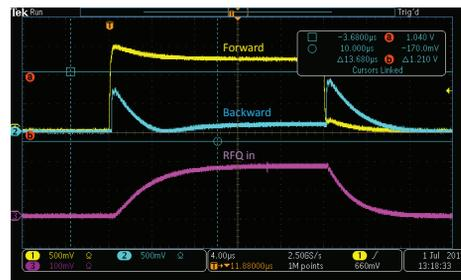
Figure 5: Forward, reflection wave and pick-up power in RFQ with nominal power of 5 kW.
