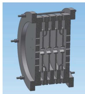
Figure 9: Design of DAW cell cold model.
