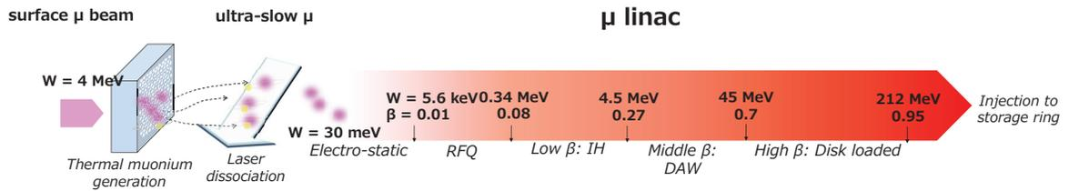
Figure 1: Configuration of low-emittance muon beam.
