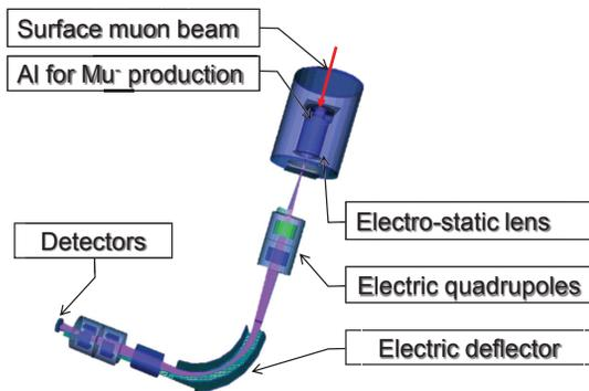
Figure 2: Setup of the SOA lens commissioning.
