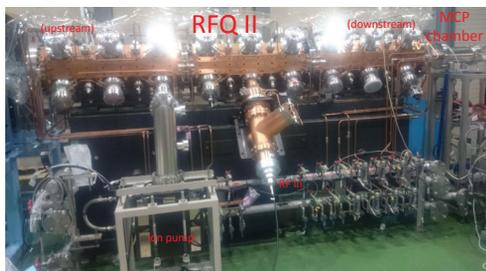
Figure 4: Photo of the RFQ offline test at the J-PARC LINAC building.
