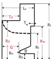
Figure 7: Two dimensional model of the DAW cavity and notations of the dimensions. Red characters are variable parameters in the optimization process.
