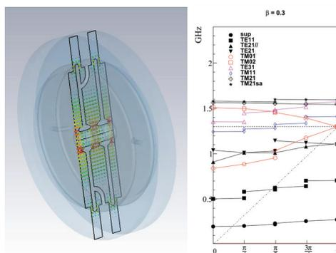
Figure 8: Dispersion curve with optimized cavity in several  $\beta$  calculated by CST MICROWAVE STUDIO.
