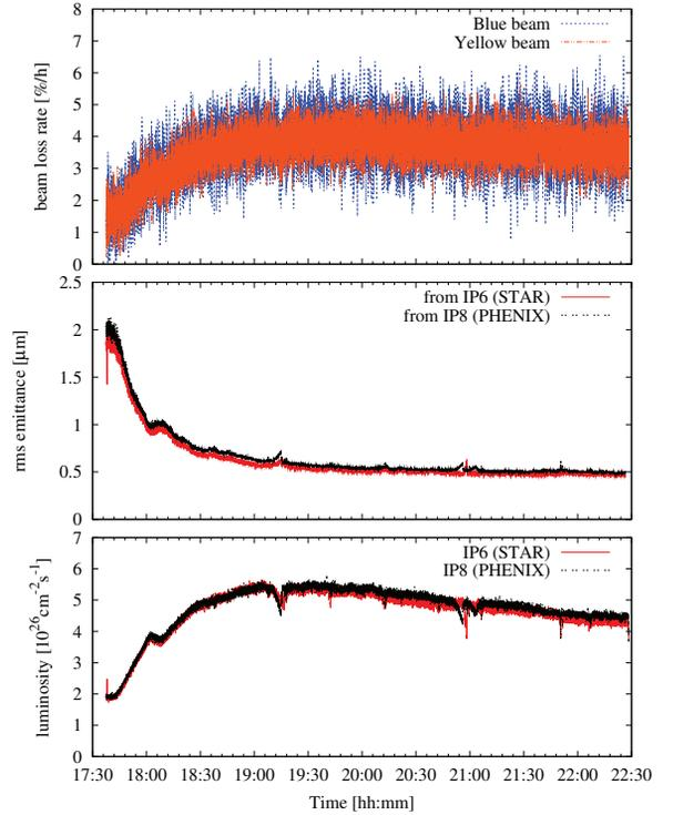
Figure 1: Au+Au store (fill 18196) with relative beam loss rates (a), normalized rms emittances calculated from luminosity and intensity (b), and luminosities at the STAR and PHENIX experiments (c). The reduction in the emittances and the corresponding increase in the luminosity are due to stochastic cooling during store.
