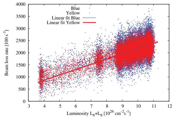
Figure 2: Blue and Yellow beam loss rates as a function of the total luminosity  $\mathcal{L}_6 + \mathcal{L}_8$  for fill number 18196. The units for the luminosity and beam loss rates are chosen so that the linear fit coefficient is returned in units of barn. Fitted values case are  $\sigma_{tot} = (216.02 \pm 0.31)$  barn for Blue, and  $\sigma_{tot} = (213.25 \pm 0.21)$  barn for Yellow. The error is the statistical standard error.
