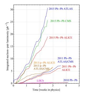
Figure 6: Nucleon-nucleon integrated luminosity in each experiment in all LHC heavy-ion runs to date [1, 12, 13], from the first declaration of Stable Beams.
