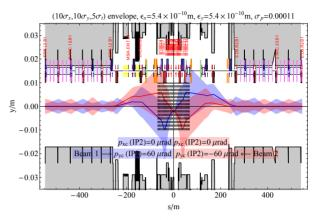
Figure 1: Vertical beam envelopes around the ALICE experiment in physics conditions with spectrometer bump angle  $-77 \mu$ rad, external bump  $+137 \mu$ rad for Beam 1.
