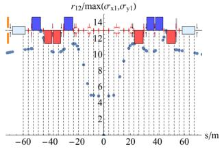
Figure 2: Beam-beam separation in units of the larger horizontal/vertical beam size close to ALICE. Vertical lines represent possible encounter points.
