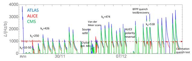
Figure 3: Luminosity for 3 of the 4 experiments, during the 2015 Pb-Pb run showing the progressive increase of stored bunch number  $k_b$  and the various interruptions of regular data-taking. The dashed line shows the design luminosity [3].
