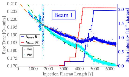
Figure 1: Bare tune evolution at the injection plateau for Beam 1 in fill 4526, overlaid with beam intensities.
