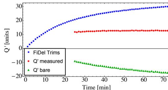
Figure 4: Example of  $Q'$  decay during the injection plateau.
