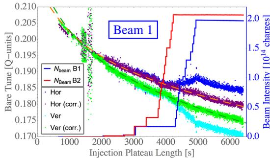
Figure 2: Fig. 1 overlaid with the tune evolution corrected for intensity effect. Orange and green dashed lines show fits to purple (hor.) and green (ver.) points.
