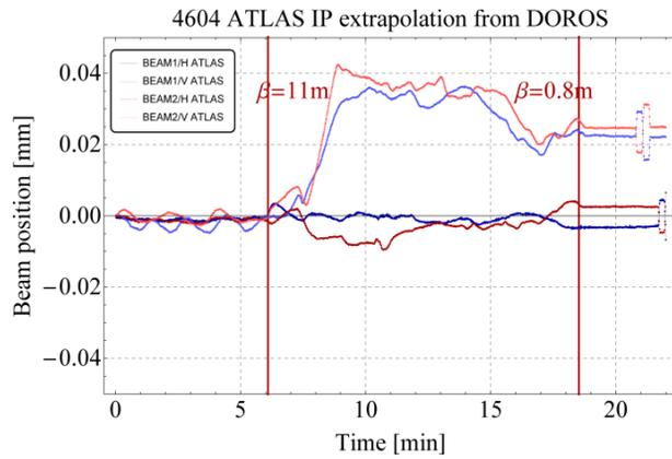
Figure 4: Evolution of the beam positions in ATLAS obtained by extrapolation of the DOROS data in fill 4604.
