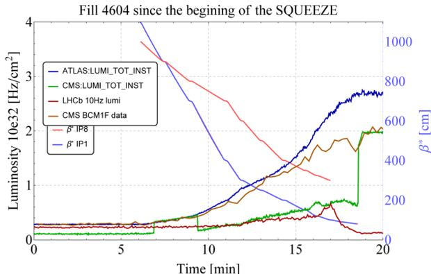
Figure 1: The evolution of luminosity and  $\beta^*$  for the three IPs with collisions (ATLAS, CMS and LHCb) in the last MD. The 'jumps' of the CMS luminosity were caused by the calibration of the luminometer.
