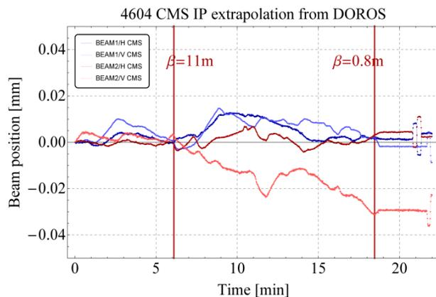
Figure 5: Evolution of the beam positions in CMS obtained by extrapolation of the DOROS data in fill 4604. A separation (of about  $1.5\sigma$ ) developed close to the beginning of the squeeze, mainly driven by a beam 2 vertical drift.
