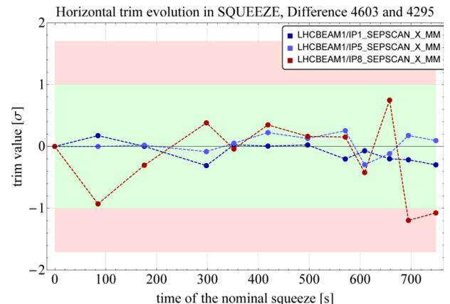
Figure 3: Horizontal luminosity corrections applied in November 2015 in unit of beam size as a function of the time along the squeeze w.r.t. to the settings established in August 2015.
