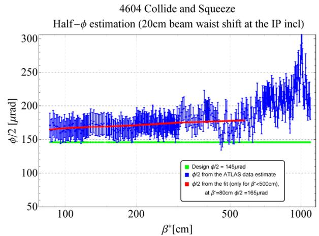
Figure 6: The estimate of the crossing angle ( $\phi/2$ ) versus  $\beta^*$  for IP1 during the LHC fill 4604.
