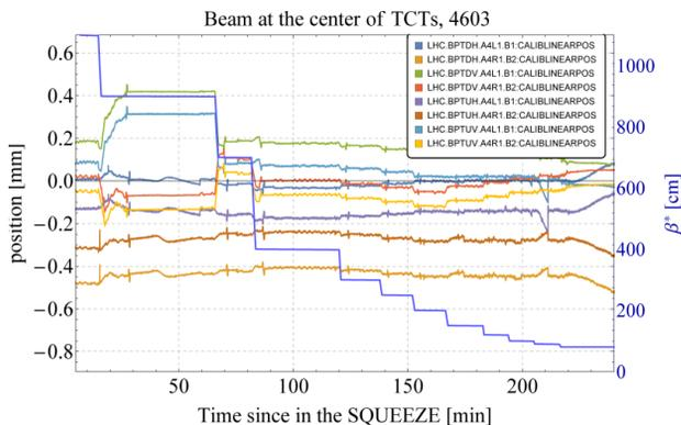
Figure 2: Example of orbit evolution at the TCTs in IP1 (ATLAS) during one of the squeeze tests with colliding beams. The position is recorded by beam position monitors embedded into the collimator jaws.
