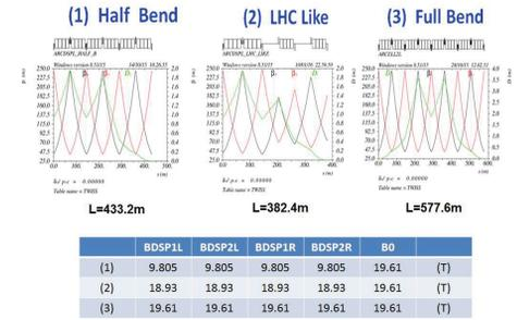
Figure 5: Dispersion suppressor section for SPPC.
