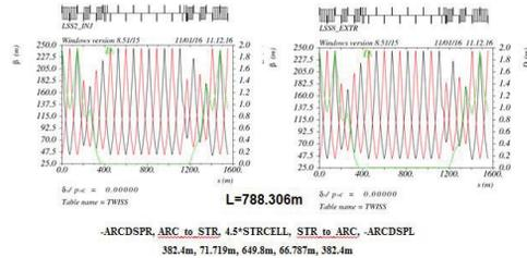
Figure 9: Long straight section for injection and extraction.
