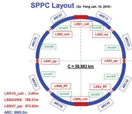
Figure 1: SPPC lattice layout.
