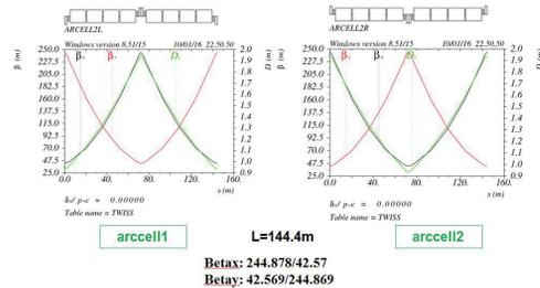
Figure 3: SPPC FODO cell optics.
