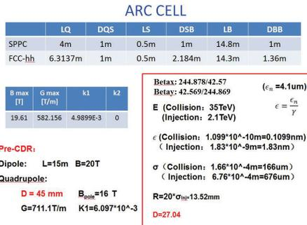
Figure 2: SPPC FODO cell parameter choice.
