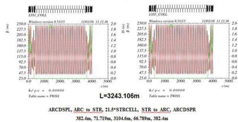
Figure 7: Long straight section for collimation.
