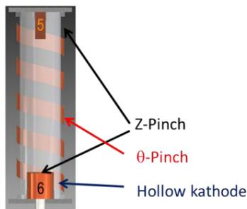
Figure 2: Schematic drawing of the Linear Screw Pinch.
