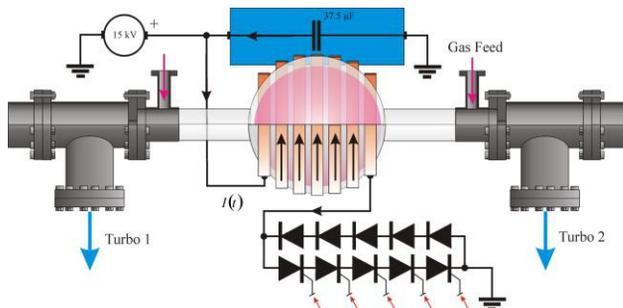
Figure 1: Experimental set-up of the Theta Pinch plasma including differential pumping system [8, 9].
