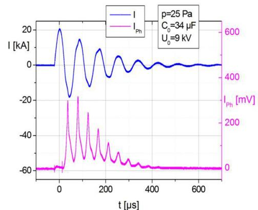
Figure 3: Current and ignition behaviour of the Spherical Theta Pinch plasma [8].
