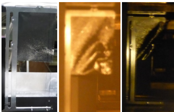
Figure 6: Fifth carbon foil after (left-right) 0, 29 and 88 mAh
