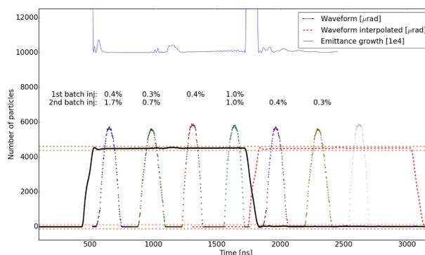
Figure 3: Calculated emittance growth due to kicker waveform ripple.
