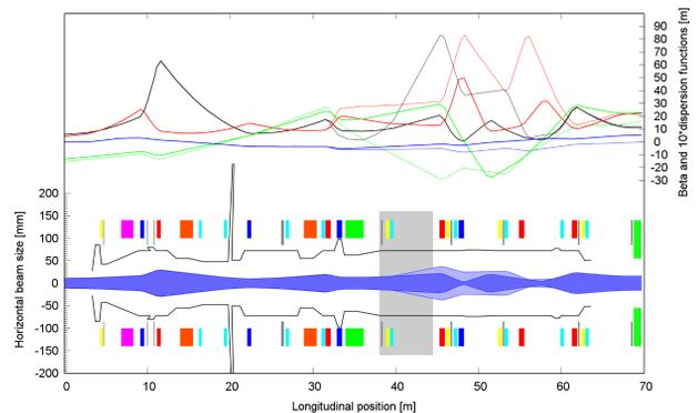
Figure 2: Present (thin) and new (thick) optics for the PSB to PS transfer in the top part. Horizontal betatron and dispersion functions are denoted in black and green, vertical betatron and dispersion functions in red and blue, respectively. In the bottom part the  $3\sigma$  horizontal LHC beam envelope is shown.
