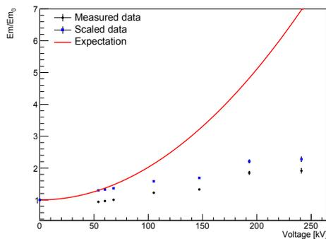
Figure 4: Measured emittance growth from PS injection kicker deflections on extraction flattop. In red the analytical expectation of emittance growth for the applied kicks.
