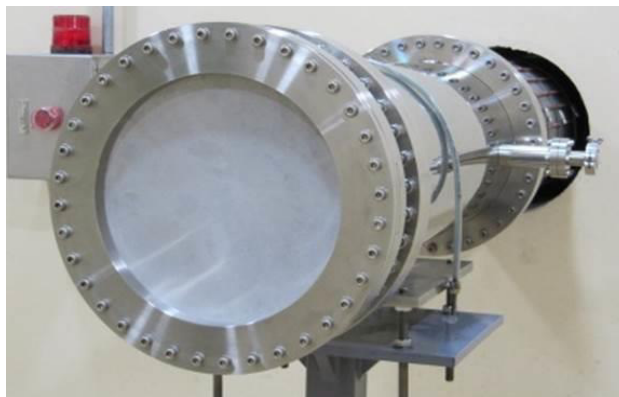
Figure 7: AlBeMat beam window at the end of beamline.
