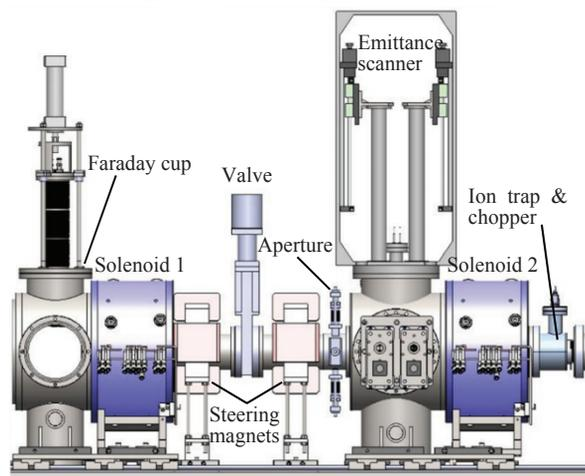
Figure 1: Layout of the Low Energy Beam Transport line (LEBT) of XiPAF.
