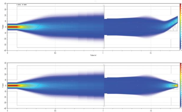
Figure 6: Beam envelop in y direction with chopper (up) and without chopper (down).
