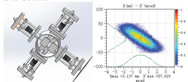
Figure 4: Primary structure of the aperture (left) and particles distribution at the RFQ entrance with the Aperture (right).
