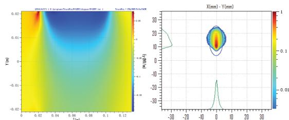
Figure 5: The electric field of the chopper in y direction (left), chopped beam spot at the LEBT exit (right)
