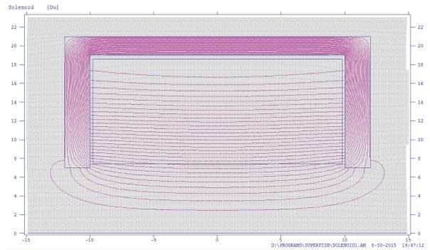
Figure 2: Magnetic field distribution of the solenoid calculated by the SUPERFISH code.
