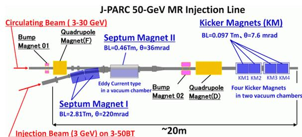
Figure 1: The schematic of the Injection Magnets group in MR.
