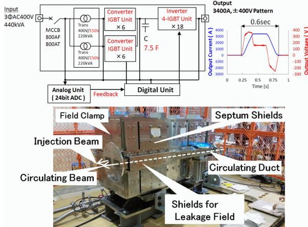
Figure 2: The diagram of the new power supply(Upper). The photograph of the new magnet(Lower).
