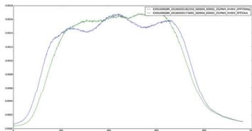
Figure 6: Overall spill for 253 Me downsampled and further smoothed. The green curve represents the intensity without the implementation of filamentation, whilst the blue curve uses filamentation.
