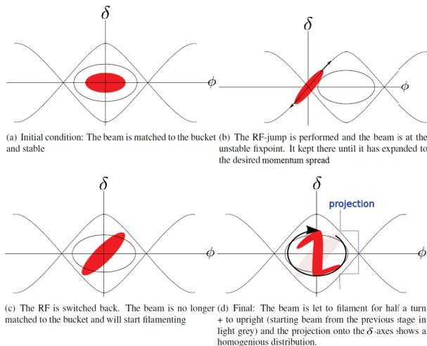
Figure 1: General scheme of a phase jump [2].
