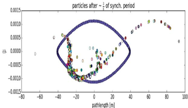
Figure 8: Particle distribution in longitudinal phase space when a phase offset was present before the phase jump.
