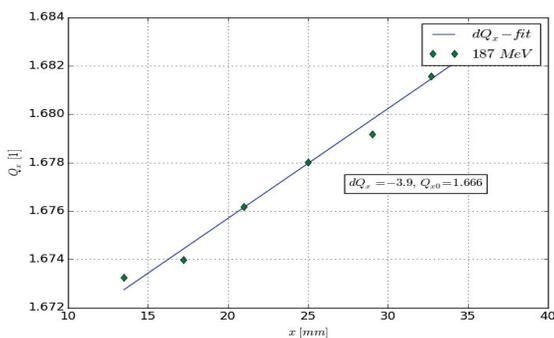
Figure 3: Horizontal chromaticity measurement for 187 MeV, vertical axis shows the measured horizontal tune and the horizontal axis shows the beam position at the maximum dispersion position.
