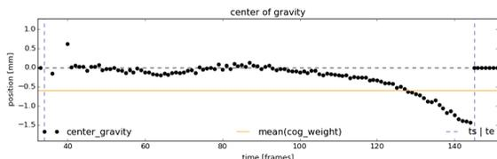
Figure 7: horizontal position position measurement in a region of the HEBT with  $D \neq 0$ .
