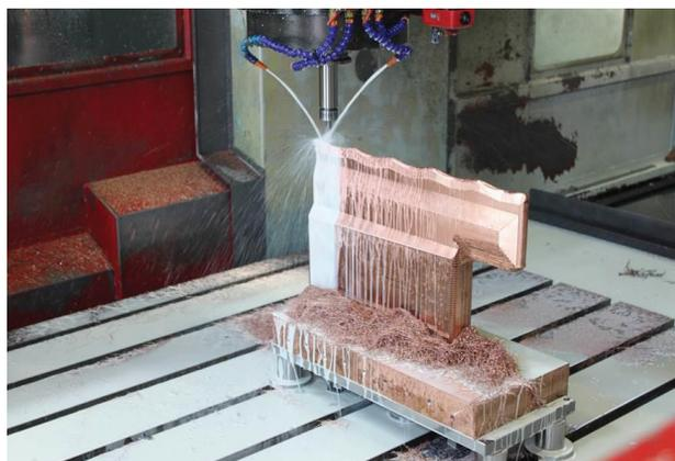
Figure 3: Modulation machining with the ball-end mill.
