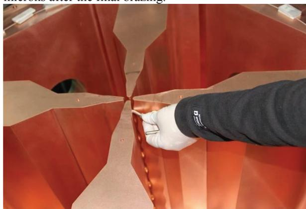
Figure 5: Alignment of segments by using pin gauges.
