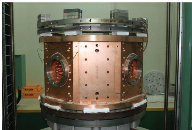
Figure 4: RFQ unit module just before the brazing.
