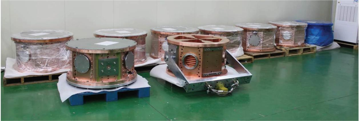
Figure 6: Fabricated nine unit modules of RISP RFQ.
