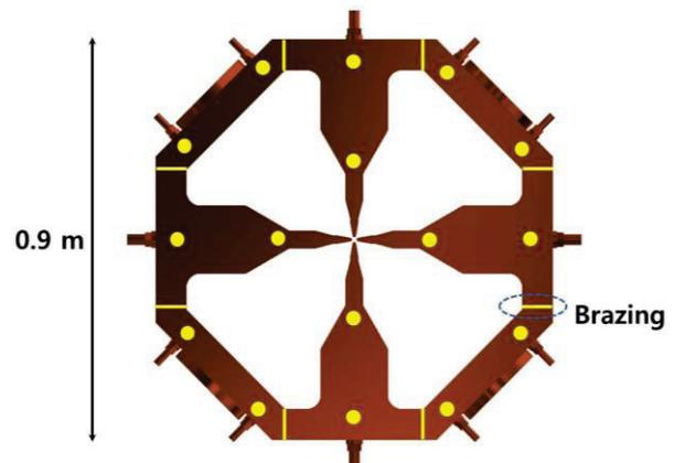
Figure 2: Cross sectional view of the cavity.
