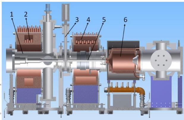
Figure 2: E-gun – collector test bench (1 – e-gun, 2 – e-gun coil, 3 – vacuum valve, 4 – collector coil, 5 – drift tube, 6 – electron collector).
