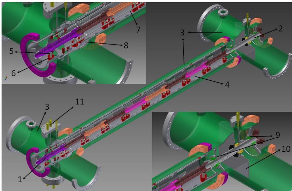
Figure 1: 3D model of RAON EBIS CB DT section (middle), zoomed e-gun side (upper-left), zoomed collector side (lower-right) (1 – DT1, 2 – DT10 (8 DTs are placed between DT1 and DT10), 3 – vacuum chambers, 4 – scaffold, 5 – ceramic standoff, 6 – protection cup, 7 – potential lead, 8 – NEG strip, 9 - DT10 support and alignment fixture, 10 – differential pumping baffle, 11 – HV feedthrough).
