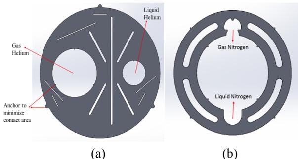
Figure 2: (a) Helium Spacer, (b) Nitrogen Spacer.
