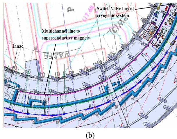
Figure 1: (a) Multichannel line to SRF valve box, (b) Multichannel line to superconductive radio frequency cavities.
