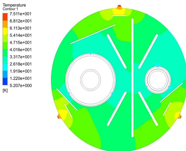
Figure 6: Temperature distribution of spacer.
