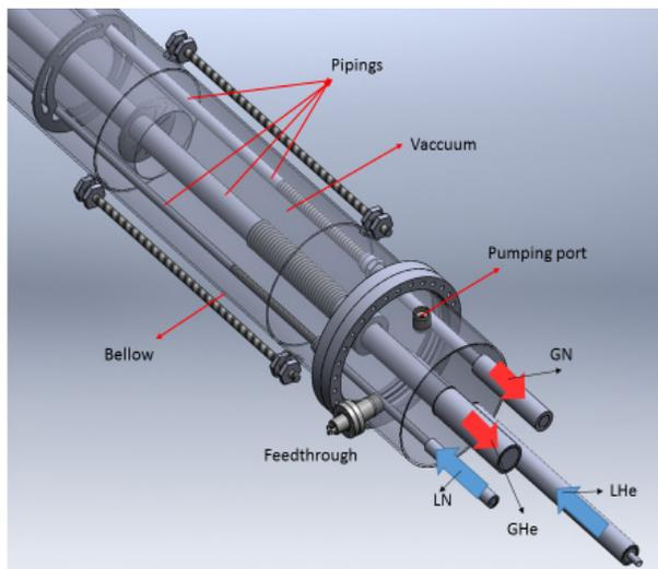
Figure 4: Detachable Multichannel line.
