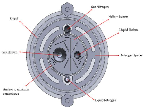
Figure 3: A Sectional View of NSRRC Multichannel line.
