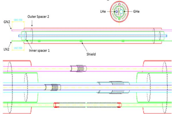
Figure 5: Connecting pipes with Anti-Torque Bellow.
