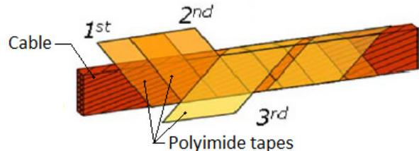
Figure 1: Superconducting cable insulation [2].
