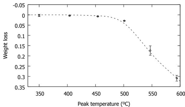
Figure 5: Weight loss of polyimide tape vs peak temperature. The dashed line is given by the model, the round markers are the average of the weight loss measured after the heat treatment with their standard deviation.
