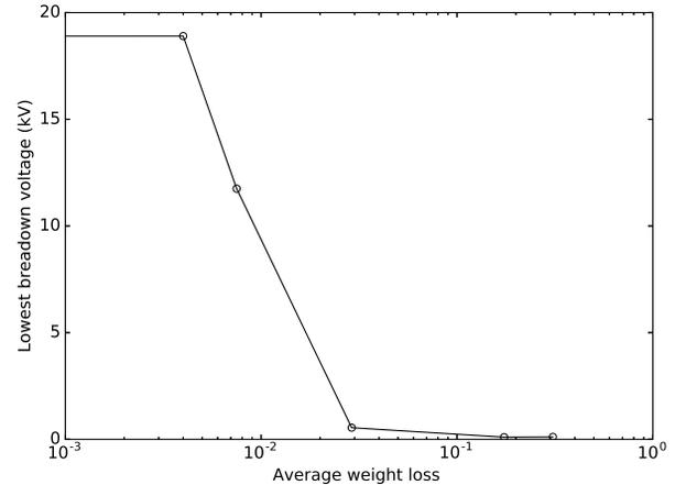
Figure 6: Lowest breakdown voltage measured on cable stacks vs average weight loss of polyimide tape measured after heat treatment.
