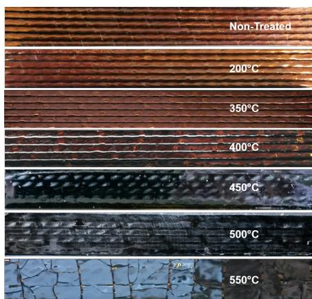
Figure 3: Cable stacks (side view) before and after the heat treatment with different peak temperatures
