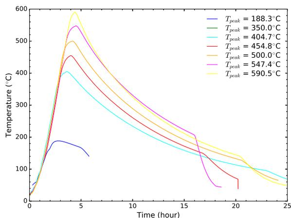
Figure 2: Temperature profiles of the cable stacks during the heat treatment.
