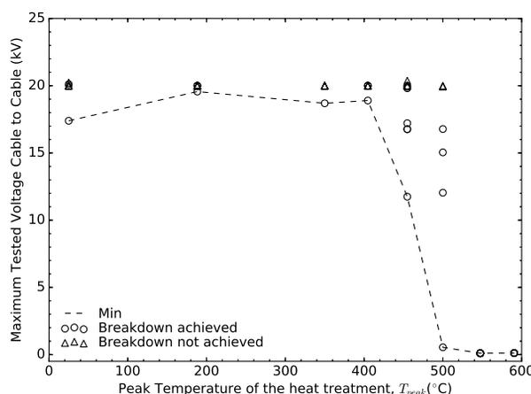
Figure 4: Results of the dielectric strength measurements after heat treatments at different peak temperature
