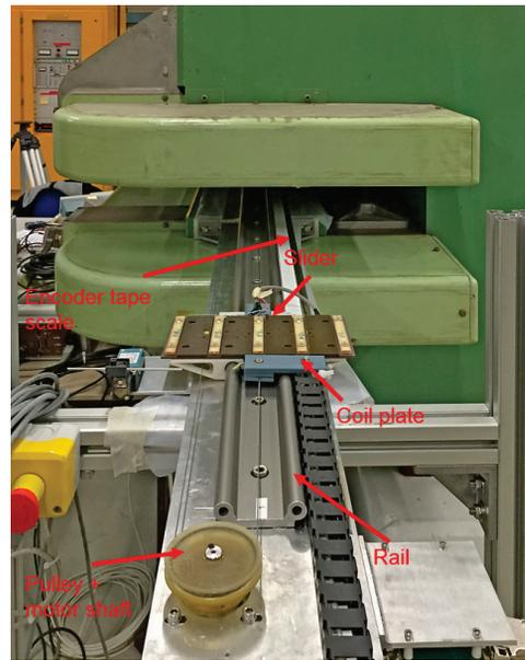
Figure 2: The prototype version of the translating fluxmeter installed on CERN's reference dipole for magnetic measurements.
