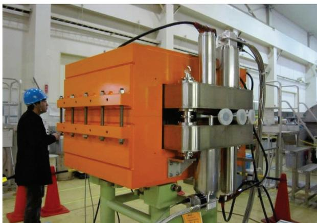
Figure 2: HTS switching magnet from downstream.
