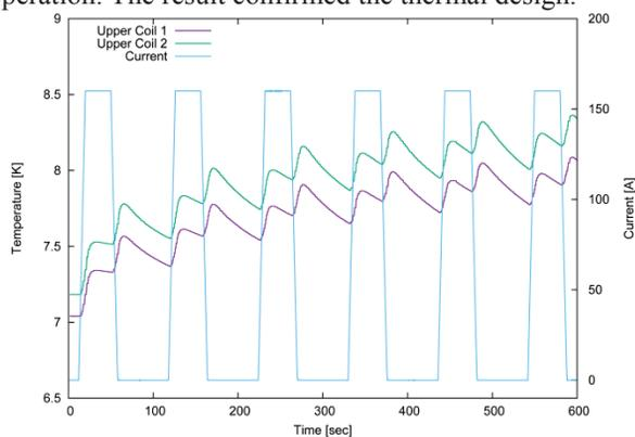
Figure 5: Temperature of upper coil during pattern operation.
