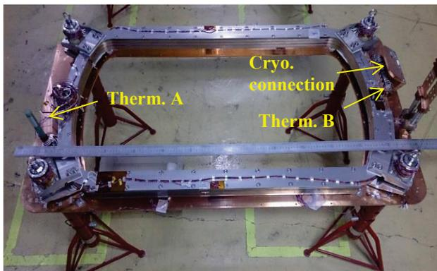
Figure 3: Upper coil assembly without thermal shields.
