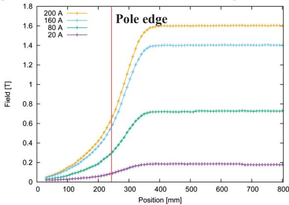
Figure 7: Field distribution for each excitation level.
