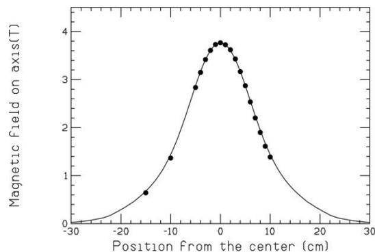
Figure 1: Field distribution along the axis. The solid line shows results of the simulation by TOSCA.
