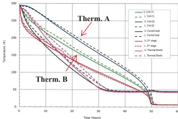
Figure 4: Initial cooling performance of the HTS magnet.
