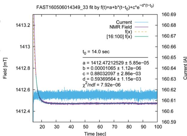
Figure 9: Field strength after excitation with cycling.
