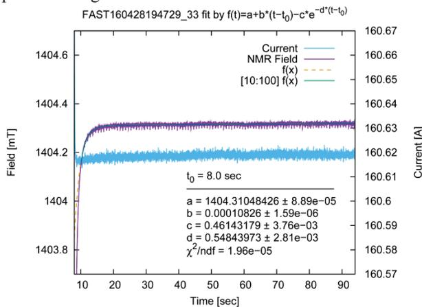
Figure 8: Field strength after excitation without cycling.
