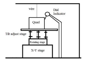
Figure 4: improved setup for Quadrupoles with large tilt angle
