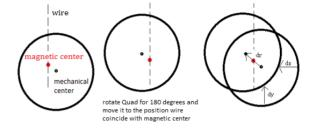
Figure 1: Rotating 180 degrees method for measurement.
