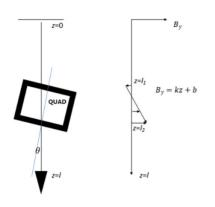
Figure 2: Rotating 180 degrees method for measurement.
